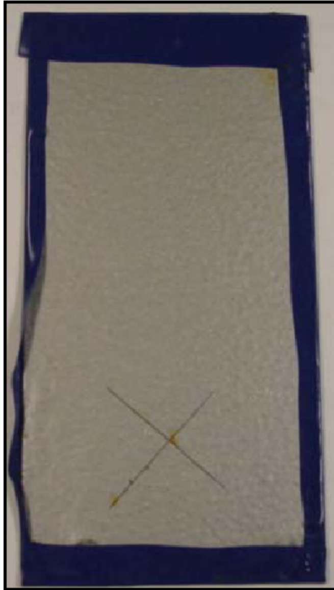
Figure 8: Sample 18 after salt spray exposure
