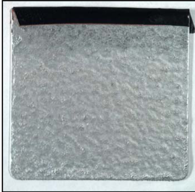
Figure 14: Sample 24 after xenon arc weathering
